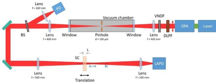
Figure 2. Scheme of the experimental setup.
